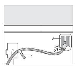
Unclip the drain hose from clips (1) and (2).
